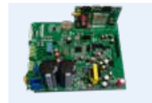
Solar Inverter PCBs
